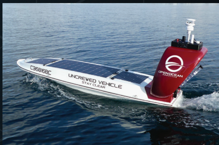
An Iridium-equipped Unmanned Surface Vessel. Photo Credit: Open Ocean Robotics
