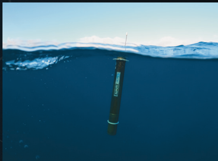
An Iridium-equipped - renewable-energy variable buoyancy profiling float. Photo Credit: Seatrec Inc
